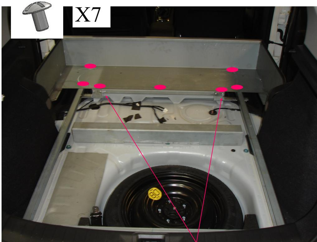
RENTRE L'ARRET de CHARGE DANS LE VEHICULE PUIS FIXÉ LE AVEC 7 VIS POELIER M6 LG 10 DANS LES CLIPS ECROU EN ATTENTE.
