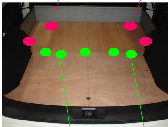
FIXER LE PLANCHER AVEC 5 VIS Ø3.9 x 25 AUTOFORANTE EN SE SERVANT DES TROUS DANS LE PLANCHER COMME GABARIT ●
