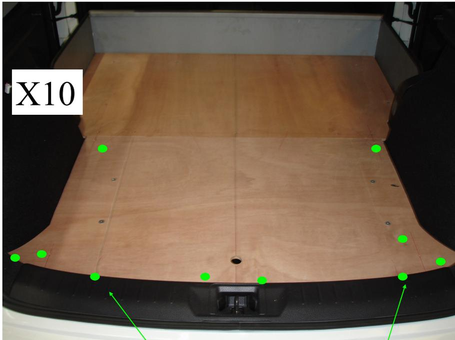
FIXER LES PLANCHERS ARRIERE AVEC 10 VIS Ø3.9 x 25 AUTOFORANTE
