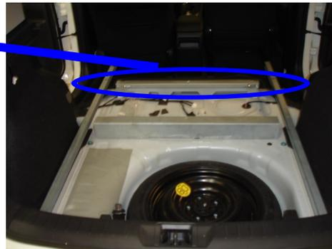
FIXER LA TRAVERSE AVANT SUR LE SUPPORT DU CHASSIS SU VEHICULE
