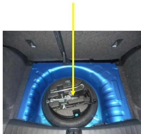
**L'HABITACLE DOIT ETRE DANS CETTE CONFIGURATION POUR MONTER L'ARRET DE CHARGE**
