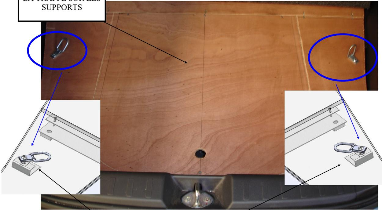
FIXER LE PLANCHER ARRIERE AVEC VIS POELIER M6 lg 25 EN
