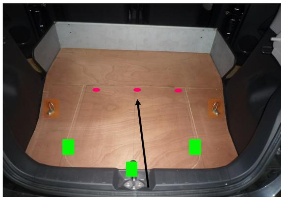
FIXER LA TRAPPE AVEC 3 VIS AUTOFORANTE 3,9x 25 ● AINSI QUE 3 VIS A BOIS 4 x 20 ■ EN SE SERVANT DES TROUS DÉJÀ PERCÉS DANS TRAPPE COMME GABARIT
