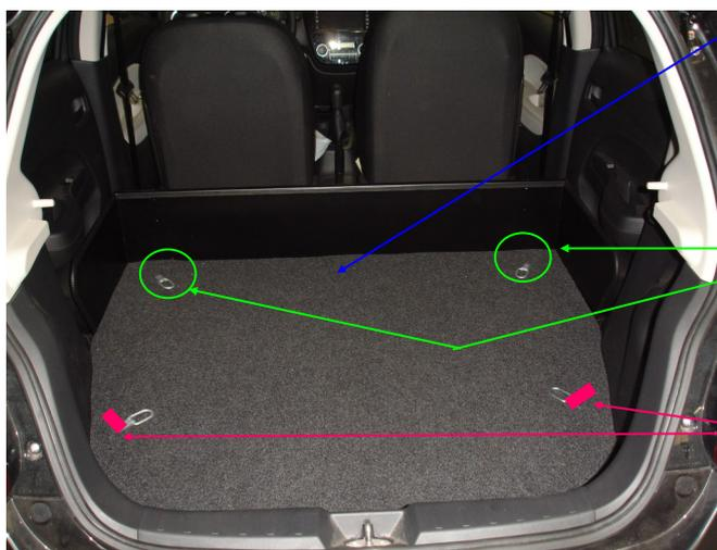
FIXER LES 2 ANNEAUX D'ARRIMAGE AVANT AVEC 2 VIS POELIER M6 Lg 25
