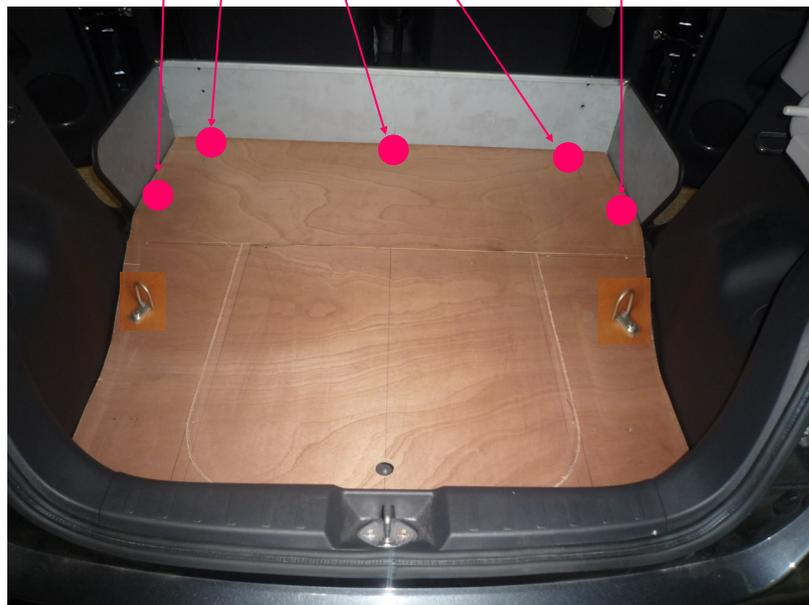
FIXER LE PLANCHER AV & AR AVEC 6 VIS AUTOFORANTE Ø3.9 x25
