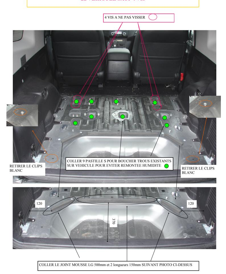
RENTRER ARRET de CHARGE PAR LA PORTE ARRIERE PUIS FIXER LE AVEC 4 VIS D'ORIGINE VEHICULE
