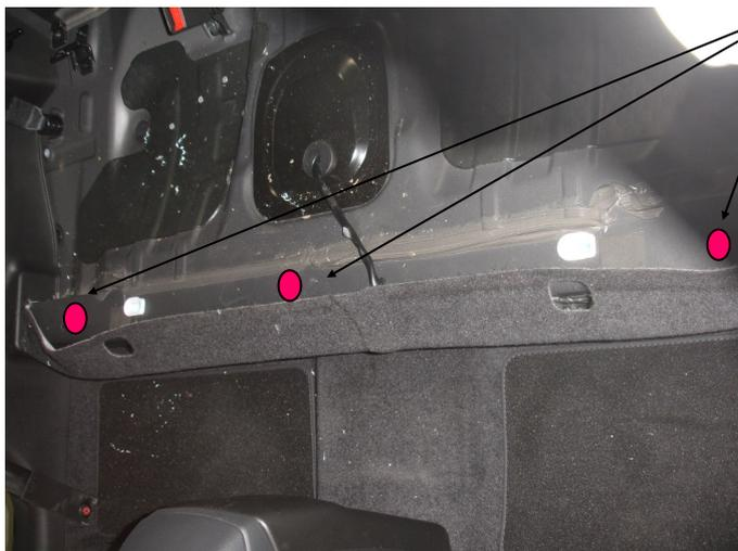
REPERER LES 3 TROUS EXISTANTS SUR CHASSIS DU VEHICULE ● POUR FIXER LA TRAVERSE AVANT REP 111 (FAIRE 2 TROUS DANS LA MOQUETTE POUR PASSAGE RIVET TETE ECLATEE)
