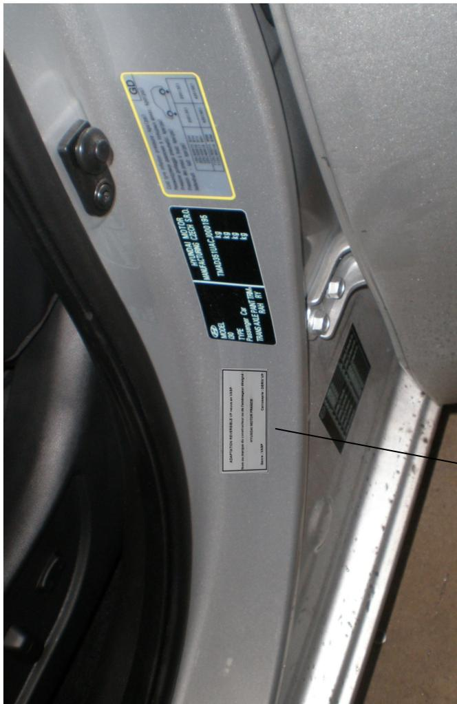
COLLER LA PLAQUE TRANSFORMEUR A COTE DE LA PLAQUE DU CONSTRUCTEUR
